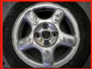
2 – Putty and reconstruct the alloy wheel if necessary, then wait a few minutes for it to dry. After sanding with P120 P240 P 400, mask with the special cards included in the kit.
